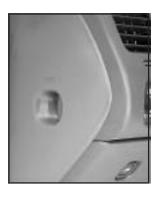
Some fuses are in a fuse block at the end of the instrument panel on the driver's side of the vehicle. Pull off the cover labeled FUSES to expose the fuses.
